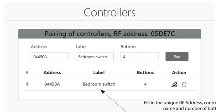
Fill in the unique RF Address, controller name and number of buttons
