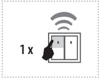
If the light is switched off, pressing the programmed button will switch it on. If the light is switched on, pressing the programmed button will switch it off.
