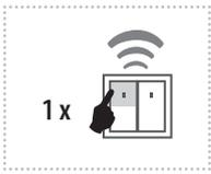
After pressing the programmed button, the light begins to illuminate in the programmed time interval in a range of 2 seconds to 30 minutes.
