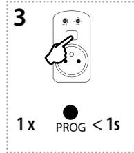
Press of programming button on socket RFDSC-71 shorter than 1 second will finish programming mode. The LED lights up according to the pre-set memory function.
