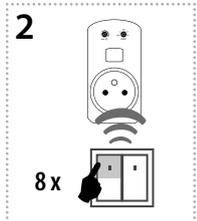
Eight presses of selected button on the RF transmitter assigns the function OFF (must be a lapse of 1s between individual presses).
