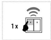
The dimmer output switches off by pressing the button.
