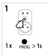
Press of programming button on receiver RFDSC-71 for 1 second will activate receiver RFDSC-71 into programming mode. LED is flashing in 1s interval.
