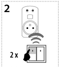
Two presses of your selected button on the RF transmitter assigns the function light scene 2 (must be a lapse of 1s between individual presses).
