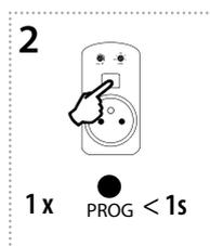
Pressing the programming button on the RFDSC-71 receiver for less than 1 second will finish the programming mode, this will reverse the memory function. The LED lights up according to the current pre-set memory function. The set memory function is saved.
