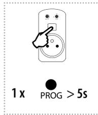
By pressing the programming button on the actuator for 5 seconds, deletion of one transmitter activates. LED flashes 4x in each 1s interval.
