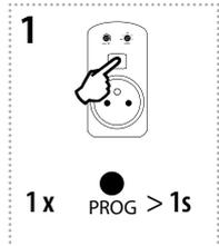
Press of programming button on actuator RFDSC-71 for 1 second will activate actuator RFDSC-71 into programming mode. LED is flashing in 1s interval.
