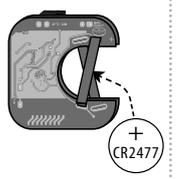
Slide a new battery CR2477 into the battery holder. Observe the polarity.
