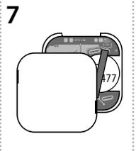
After finished programming, insert the device into the box and snap on the rear cover.
