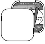
After finished programming, insert the device into the box and snap on the rear cover.
